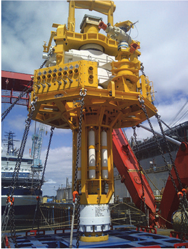
Figure V-5: Shell's Arctic oil spill containment dome (capping stack), prior to testing. (Source: Shell)
