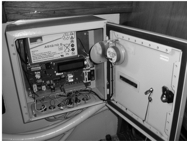
Fig. 1. The Blue Box (Control Box) of the Automated Electronic Monitoring System developed for monitoring the minke whale hunting in Norway.
